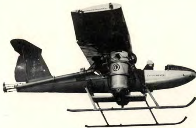
Bell's experimental, vertical-rising airplane obtains forward thrust by rotating the twin-jets 90 degrees.
