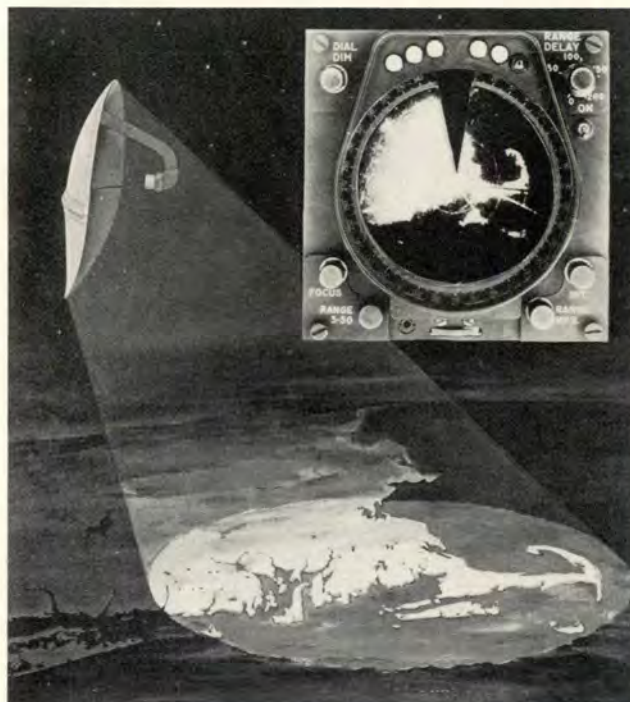
Miniature radar screen shows Cape Cod. Dark wedge at top swings to any heading for exact drift measurement.
