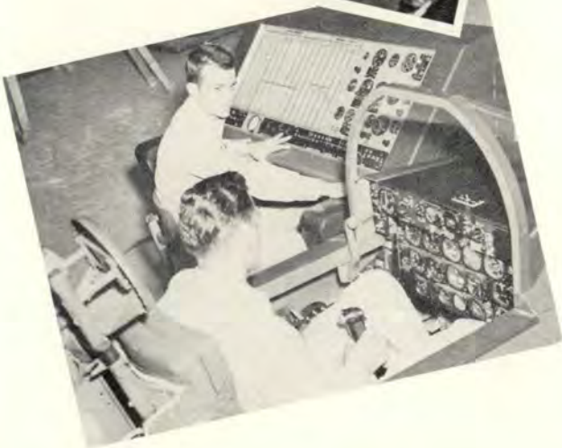
The F-84F trainer is used to teach a student complete cockpit familiarization, for practice in both normal and emergency operating procedures and to instruct in the operation of the aircraft's numerous systems.
